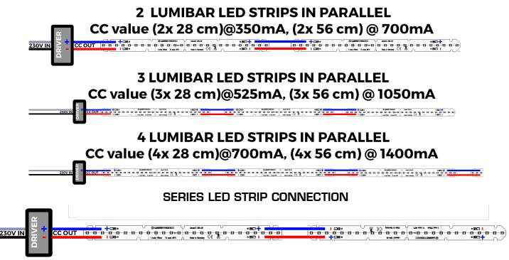
The series connection is applied by connecting the positive (+) terminal of the first LED strip to the negative (-) terminal of the second LED strip. This pattern is repeated for further LED strips, from the negative (-) of the second strip to the positive (+) of the third strip and so on. At the same time, the negative (-) of the first LED strip is wired to the (+) of the second, then the (-) of the second to the (+) of the third and so on.
