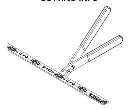
The LED strip can be separated or shortened every 83.33 mm. The connectors work on the separated parts also.
