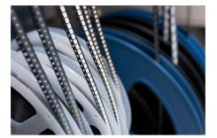
This LED strip is **made in Germany**, at a flex production line that uses the innovative manufacturing technology of plasma direct metallization, to turn flexible substrates into electrical conductive and solderable circuit boards, even those that before have not been suitable for an assembly with electronic components.
