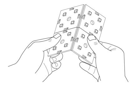
The LED module can be separated into smaller units up to 1 single module of 30x30mm. The connectors work on the separated parts also.
