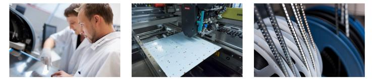
The MatrixMini is **made in Germany**, at a production line that uses the innovative manufacturing technology of plasma direct metallization, to turn substrates into electrical conductive and solderable circuit boards, even those that before have not been suitable for an assembly with electronic components.
