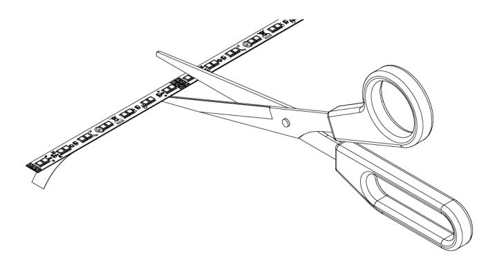
The LED strip can be separated or shortened every 100 mm. On the back of the LED strip is a double-sided heat-conducting adhesive tape, which allows installation of the LED strip. Professional LED strips can be cut with scissors.
