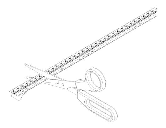
The LED strip can be separated or shortened every 10 mm. On the back of the LED strip is a double-sided heat-conducting adhesive tape, which allows installation of the LED strip. Professional LED strips can be cut with scissors.
