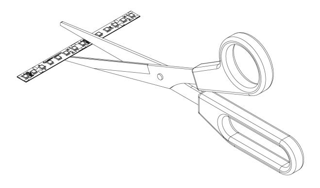
The LED strip can be separated or shortened every 100 mm. On the back of the LED strip is a double-sided heat-conducting adhesive tape, which allows installation of the LED strip. Professional LED strips can be cut with scissors.
