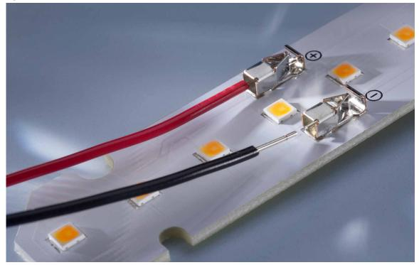
The professional LumiBar strip is connected via a solderless connection to the connection inputs provided for this purpose. The form factor and connection is Designed according to the Zhaga standard (Book 7 L28W2).
